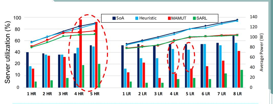
Server utilization reaching 95-97% with more types of Heterogeneous Racks (HR) to manage
